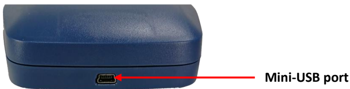
Figure 2-4: Mini-USB port on underside of Hydromette CH 17
